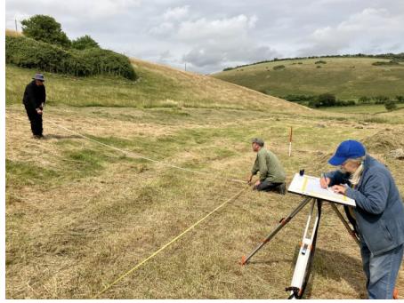
Volunteers using a plane table and tape measures to survey in the Valley of Stones with Historic England
